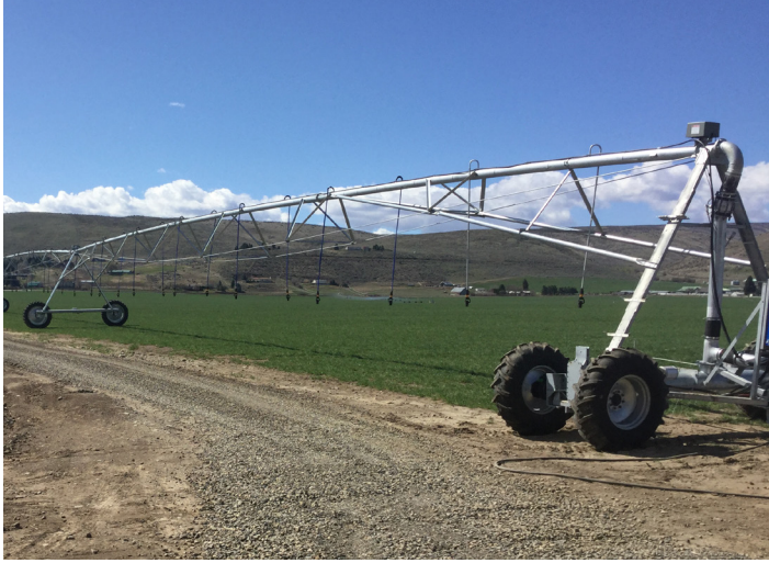
Converting rill irrigation to sprinkler irrigation systems. This improves water quality, reduces soil erosion, and enables more efficient water use. (Kittitas County Conservation District)
